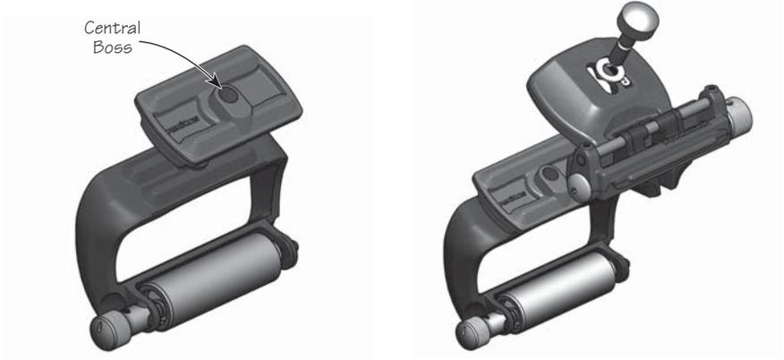
1. Orient the adapter on the roller base as shown. Note the direction of the central boss and the Veritas logo. (Discard nut.)
